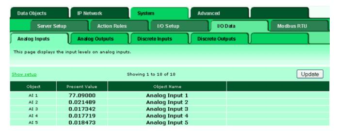
The global view of BACnet Object data is found under the Data Objects tab. This shows data from I/O points, and includes data retrieved from remote devices via the BACnet IP client or other gateway features. It also includes data generated by user programs, or written into the register by a remote client (e.g. BACnet IP client).
