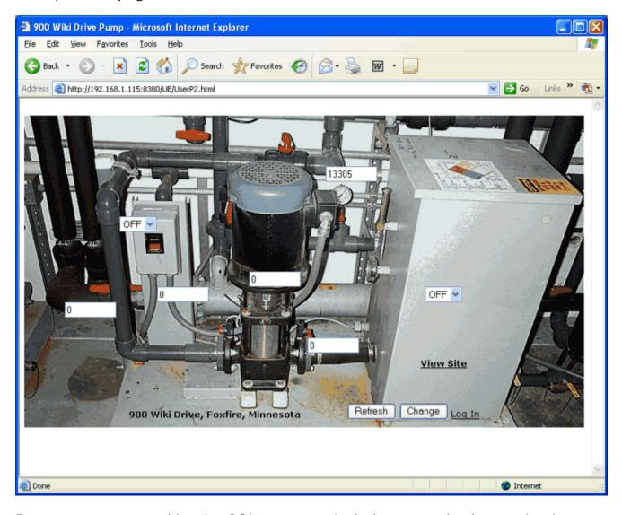
Data types supported by the CGI processor include text and select option inputs. Dynamic, live access to data is by way of object number references used as the name of the input object. Input windows can be defined as read-only. If they are not restricted, any new data entered by the user will be written into data objects.
