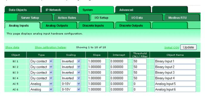
Analog inputs by default are assigned to Analog Input BACnet objects. However, if reconfigured as dry contact or discrete inputs, they are automatically reassigned to Binary Input objects.
